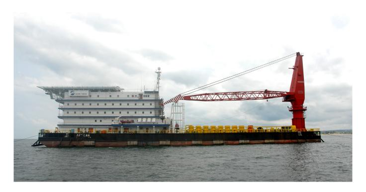
The Accommodation Support Barge provide support to production platforms and infrastructure during offshore construction or modification and maintenance. Flat bottom barges are well suited for the calm waters off the coast of West Africa.
